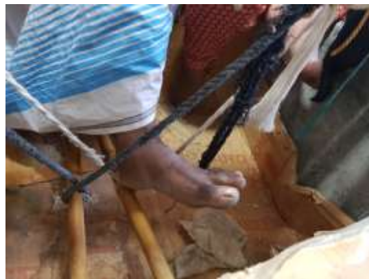
Fig 7 Paya fela, the feet technique of handloom
