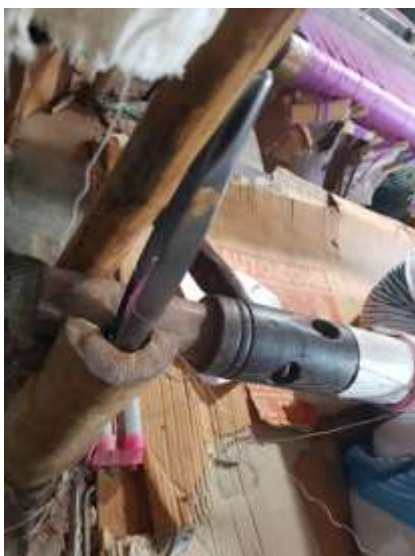
Fig 8 Muni, yarn tighter in the loom
