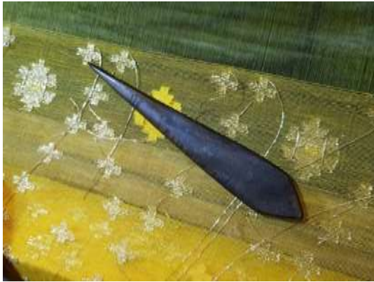
Fig 4 Chakku, equipment for weaving
